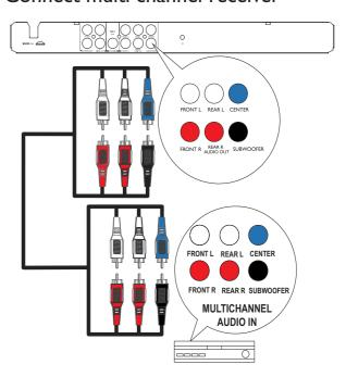
1 Connect the audio cables (not supplied) to the AUDIO OUT (FRONT L/R, REAR L/R, CENTER and SUBWOOFER) jacks on this DVD player and the audio input jacks on the device.
