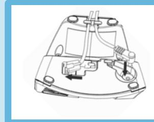
2. Connect the line cord and the power cable to their corresponding connectors at the back of the base station.
