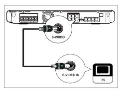
1 Connect a S-video cable (not supplied) from the VIDEO OUT-S-VIDEO socket on this unit to the S-Video input socket on your TV.
