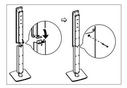
Attach the speakers to the speaker stands and secure the position with screws.
