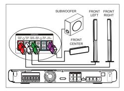
Connect the centre, front left, front right speakers and subwoofer to the matching sockets on this unit.
