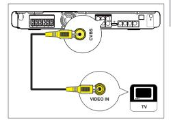
1 Connect a composite video cable (yellow supplied) from the VIDEO OUT-CVBS socket on this unit to the video input socket on your TV.
