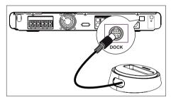
1 Connect the iPod docking station to DOCK socket on this unit.
