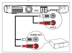
1 Connect an audio cable (not supplied) from the AUDIO IN-AUX2 sockets on this unit to the AUDIO OUT sockets on the device.
