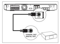
1 Connect a coaxial cable (not supplied) from the DIGITAL IN-COAXIAL socket on this unit to the COAXIAL/DIGITAL OUT socket on the device.
