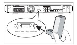
Connect the wireless transmitter to the WIRELESS TRANSMITTER socket on this unit.
