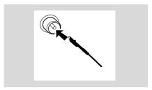
For better FM stereo reception, connect an outdoor FM antenna to the FM AERIAL (FM ANTENNA) terminal.
