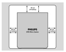
The ventilation should not be impeded by covering the ventilation openings with items, such as newspapers table-cloths, curtains, etc.
