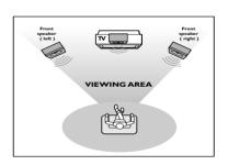
Place the front left and right speakers at equal distances from the TV set and at an angle of approximately 45 degrees from the listening position.
