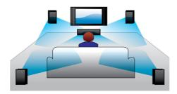
A built-in DTS and Dolby Digital decoder eliminates the need for an external decoder by processing all six channels of audio information to provide a surround sound experience and an astoundingly natural sense of ambience and dynamic realism. Dolby Pro Logic II provides five channels of surround processing from any stereo source.
