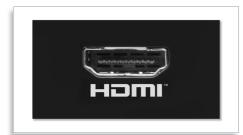
HDMI is a direct digital connection that can carry digital HD video as well as digital multichannel audio. By eliminating the conversion to analog signals it delivers perfect picture and sound quality, completely free from noise. HDMI is fully backward-compatible with DVI.
