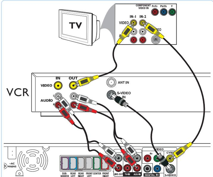
**Note:** **LINE OUT** will output sound only when the speakers volume are reduced to level 3 and below.
