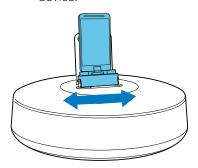
Adjust the bumpers on both sides to stabilize the portable device.
