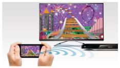
MiracastTM is a peer-to-peer wireless screencasting standard formed via Wi-Fi Direct connections. Simplified user interface likes screen-mirroring the portable device screen to bigger screen via Miracast™ certified device, no limit by pre-build codec for decoding.
