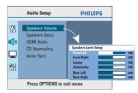
Use ◀ ► keys to set the volume level for each speaker (-6dB ~ +6dB) and press OK to confirm. 6 Use ▲▼ keys to highlight { Speakers Delay } and press ▶.
