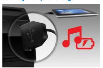
The new Philips Universal USB charging interface supplies 1 Amp of current to a smart device, which is sufficient enough to charge its battery and power it up for intensive use. The software protocol is also designed to be universally compatible with virtually all smart phones available in the market and starts the charging process instantly when USB is connected.
