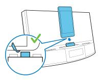
2 If necessary, rotate the USB connector on the docking system, and then place your Android-powered phone into the dock.
