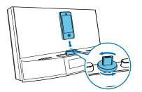
3 Adjust the bumpers on both sides of the connector to stabilize the phone.
