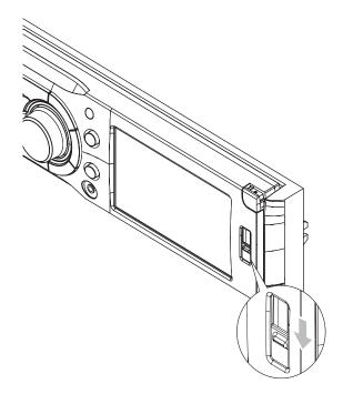
Insert the USB device into the USB socket.
