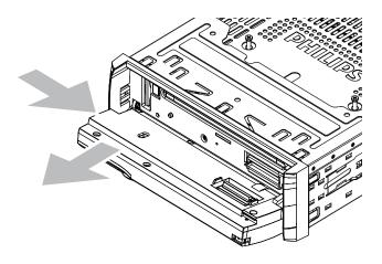
3 Take off the panel and store it in the supplied carry case to protect it from dirt or damage.
