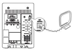
1 Connect the supplied MW antenna to the MW AERIAL socket.
