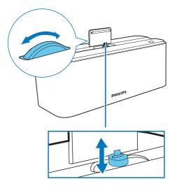
4 Slide the connector to place your device in the middle of the docking speaker.
