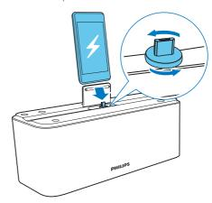
3 Adjust the wheel on the back of the connector to stabilize the device.
