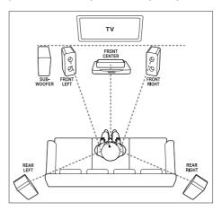
Surround sound depends on factors such as room shape and size, type of wall and ceiling, windows and reflective surfaces, and speaker acoustics. Experiment with the speaker positions to find the optimum setting for you.
