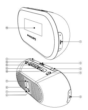
(1) + TUNING -Tune to radio stations REPEAT ALARM/BRIGHTNESS CONTROL (2) Repeat alarm. Adjust display brightness. (3) AI 1/AI 2 Set alarm. Activate/deactivate alarm timer. (4) ①/SOURCE Turn on/off the unit Select a source: FM/DAB tuner or MP3 link. (5) - Volume + Adjust volume. (6) Battery compartment (7) **FM ANT** Improve FM reception. (8) DC 5V Connect power.
