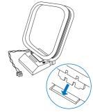
2 Connect the AM loop antenna to the AM jack on the back of the main unit.
