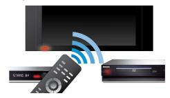
EasyLink lets you control multiple devices like DVD players, Blu-ray players, soundbar speakers, Home theatre systems and TVs etc. with one remote. It uses HDMI CEC industry-standard protocol to share functionality between devices through the HDMI cable. With one touch of a button, you can operate all your connected HDMI CEC-enabled equipment simultaneously. Functions like standby and play can now be carried out with absolute ease.
