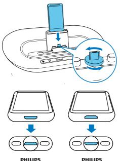
**3** Adjust the bumpers on both sides of the connector to stabilize the phone.
