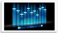
This parametric equalizer provides 11 different frequency bands (63 Hz, 100 Hz, 160 Hz, 250 Hz, 400 Hz, 630 Hz, 1 KHz, 2 KHz, 4 KHz, 8 KHz and 16 KHz), giving you the freedom to adjust bass, midrange and treble to suit the acoustics of your car. What's more, the equalizer allows you to save your favourite equalisation settings, and to recall them easily. With Philips, you will always enjoy fabulous incar sound the way you want it, anytime you want it.
