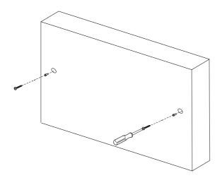
4 Secure the wall mount bracket onto the main unit with 2 supplied screws.
