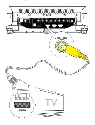
If yourTV connected to a set-topbox (to convert analog signal into digital signal), connect the supplied AV cable to AV output sockets on the set-top-box and the AV1 IN or AV2 IN sockets.
