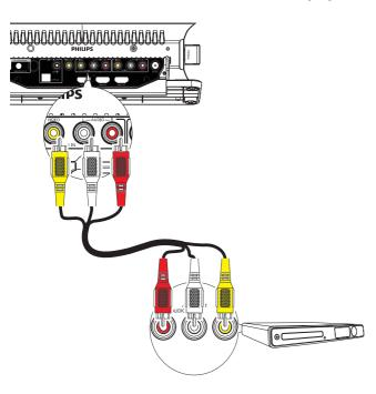
You can also connect the supplied AV switch cable to the AV FRONT socket first, then connect the AV cable to the AV output sockets on the DVD player.
