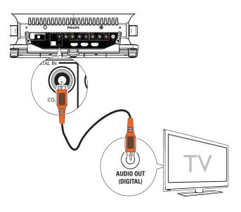
You can also connect the system to the TV by using the supplied AV cable (see below illustration).
