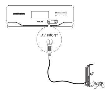
You can connect the AV output sockets on a game console to the AV1 IN or AV2 IN sockets on the system.
