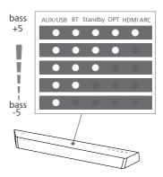
3 Press - Treble + Press -Treble + on the remote control to increase/decrease Treble's volume.
