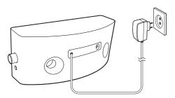
Connect the AC power cord to the wall power socket.
