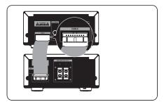
Connect the control cable between the player and amplifier.
