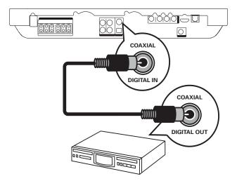
1 Connect a coaxial cable (not supplied) to the **DIGITAL-IN-COAXIAL** jack on this Home Theater System and the COAXIAL/DIGITAL output jack on the device.
