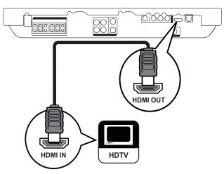
1 Connect the HDMI cable to the HDMI OUT jack on this Home Theater System and the HDMI input jack on the TV.
