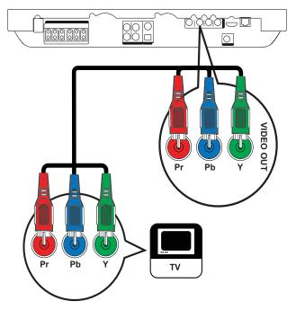
1 Connect the component video cable (not supplied) to the **Y Pb Pr** jacks on this Home Theater System and the COMPONENT VIDEO input jacks on the TV.
