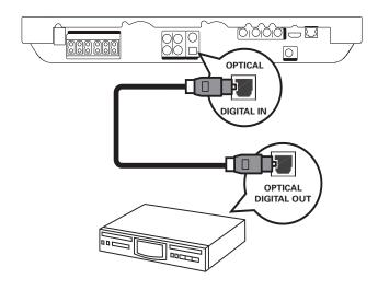
1 Connect an optical cable (not supplied) to the **DIGITAL-IN-OPTICAL** jack on this Home Theater System and the OPTICAL/SPDIF output jack on the device.
