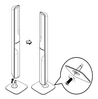
1 Attach the speakers to the speaker stands and secure the position with screws.
