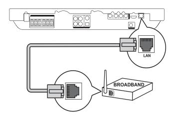
1 Connect the network cable (not supplied) to the LAN jack on this Home Theater System and the LAN jack on the broadband modem or router.
