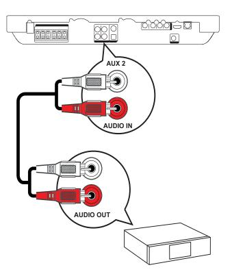
1 Connect the audio cables (not supplied) to the AUDIO IN-AUX2 jacks on this Home Theater System and the AUDIO output jacks on the device.
