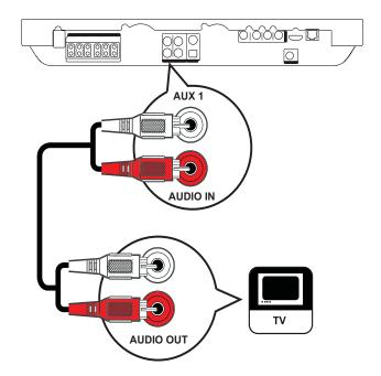
1 Connect the audio cables (not supplied) to the AUDIO IN-AUX1 jacks on this Home Theater System and the AUDIO output jacks on the TV.
