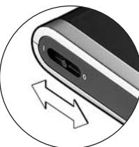
**Tip** Always switch off the Control Panel during transport to avoid the activation of the touchscreen and battery draining.
