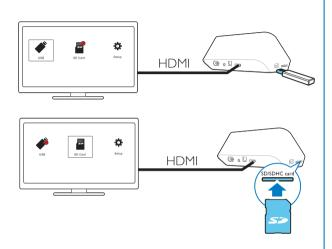
When the USB device or SD/ SDHC card is recognized by HMP4000, ♣ changes to ♣ or ■ changes to ■ on the Home screen.
