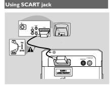
Use the SCART cable (black) to connect the DVD Player's SCART jack (SCART OUT) to the corresponding Scart input jacks on the TV (cable not supplied).
