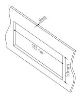
5 Install the sleeve into the dashboard and bend the tabs outward to fix the sleeve.
