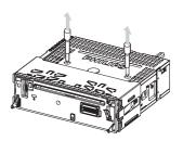
3 Remove the mounting sleeve with the supplied disassembly tools.
