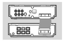
Connect the serial port marked "CONTROL CABLE" at the rear of the DVD player to the same port at the rear of the power amplifier with the supplied flat control cable.
