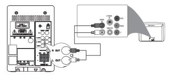
1 Connect an audio cable (red/white ends) to the audio input sockets on an audio device.
