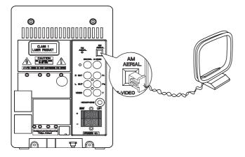
1 Connect the supplied MW antenna to the MW AERIAL socket.
