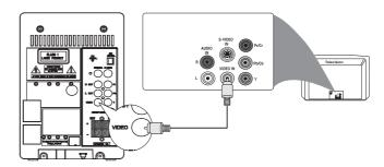
1 Connect a composite vide cable (yellow) to the composite video input socket on the TV.
