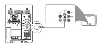
1 Connect an S-video cable (not supplied) to the S-Video input socket on the TV.
