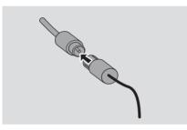
**Note:** If you are using a cable antenna system or an outdoor antenna, fit the antenna plug, instead of the wire antenna, to FM ANTENNA.
