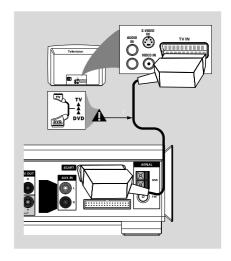
Use the SCART cable (black) to connect the DVD Player's SCART jack to the corresponding Scart input jacks on the TV (cable not supplied).
