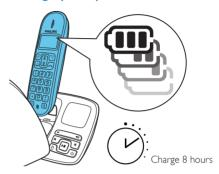
Place the handset on the base station to charge the handset. When the handset is placed correctly on the base station, you hear a docking sound.
