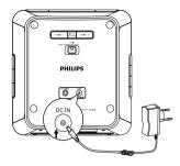
2 Connect the other end of the AC adaptor to the wall outlet.
