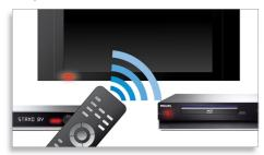
EasyLink lets you control multiple devices with one remote. It uses HDMI CEC industry-standard protocol to share functionality between devices through the HDMI cable.
