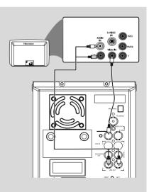
Use the composite video cable (yellow) to connect the system's VIDEO jack to the video input jack (or labelled as A/V In, Video In, Composite or Baseband) on the TV set. To hear the sound of this DVD Player through your TV, use the audio cables (white/red-not supplied) to connect LINE OUT (L/R) jacks of the DVD Player to the corresponding AUDIO IN jacks on the TV.
