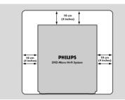
The ventilation should not be impeded by covering the ventilation openings with items, such as newspapers table-cloths, curtains, etc.
