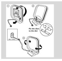
Position the antenna as far as possible from a TV, VCR or other radiation source. FM Antenna
