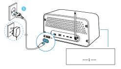
Connect the AC power cord to the **AC MAIN~** socket and then to the wall outlet.
