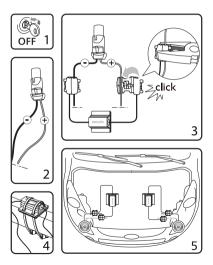
In case of re-installation of filament lamps, you may remove the Canbus as follows
