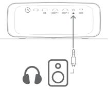
2 After connecting the speakers or headphones, press the volume control buttons on the remote control to adjust the volume to the desired level.
