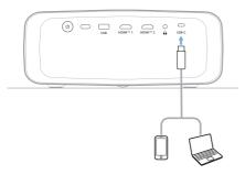
2 If the input source is incorrect, press on the remote control to bring up the input source list, and then select *USB-C*.
