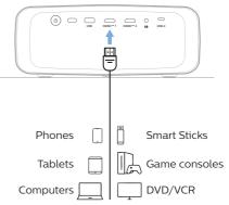
2 If the input source is incorrect, press on the remote control to bring up the input source list, and then select *HDMI1* or *HDMI2*.
