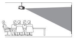
2 If the projection direction is incorrect, press on the remote control to open the settings menu, go to Projector > Install Mode > Front Ceiling and press the OK button.
