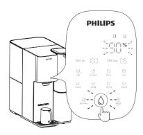
(3) When the progress reaches "90%" flashes, there is no need to empty the water. Place a container with volume no less than 2 liters under the water outlet and press " ( " . When it shows "100%", it means that the rinsing process completes.
