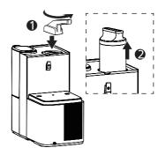
(3) Insert the new filter cartridge into the filter cartridge holder and rotate it clockwise to the locked " (2) " position, and cover the machine top lid. Put the tap water tank back to the dispenser.
