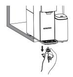
**Cleaning the air filter** (It is recommended to clean the air filter every six months to maintain the cooling performance.)
