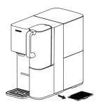
(2) Clean the air filter with clean water, wipe it dry, and reinstall it.
