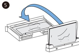
**! Carefully lay the TV set, with the screen side down, on the outer slipbox so as not to deform or damage chin at the bottom of the unit.**
