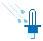
Only a burning bulb made of quartz glass (filament 2650°c, glass 800°c) can resist thermal shocks: if a drop of cold water
