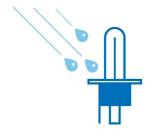
Only a burning bulb made of quartz glass (filament 2650°c, glass 800°c) can resist thermal shocks: if a drop of cold water touches the hot bulb, which can happen when you drive through water with a broken headlight unit.
