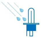
Only a burning bulb made of quartz glass (filament 2650°c, glass 800°c) can resist thermal shocks: if a drop of cold water
