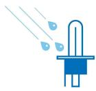
Only a burning bulb made of quartz glass (filament  $2650^{\circ}$ c, glass  $800^{\circ}$ c) can resist thermal shocks: if a drop of cold water touches the hot bulb, which can happen when you drive through water with a broken headlight unit.
