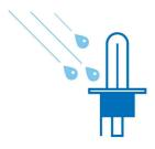
Only a burning bulb made of quartz glass (filament 2650°c, glass 800°c) can resist thermal shocks: such as, if a drop of cold water touches the hot bulb, which can happen when you drive through water with a broken headlight unit.
