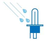
Only a burning bulb made of quartz glass (filament 2650°c, glass 800°c) can resist thermal shocks: such as, if a drop of cold water touches the hot bulb, which can happen when you drive through water with a broken headlight unit. ^Application varies per bulb type
